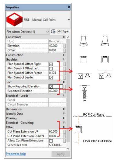
Plan Symbol Offsets and Leaders allow you to correctly document fixtures that are aligned vertically.
